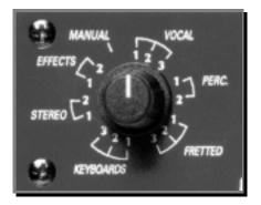
The **Presets** for the Blue Max are controlled by this sixteen position rotary encoder. As the encoder is rotated, parameters are digitally switched, simultaneously controlling attack, release, ratio and threshold.
